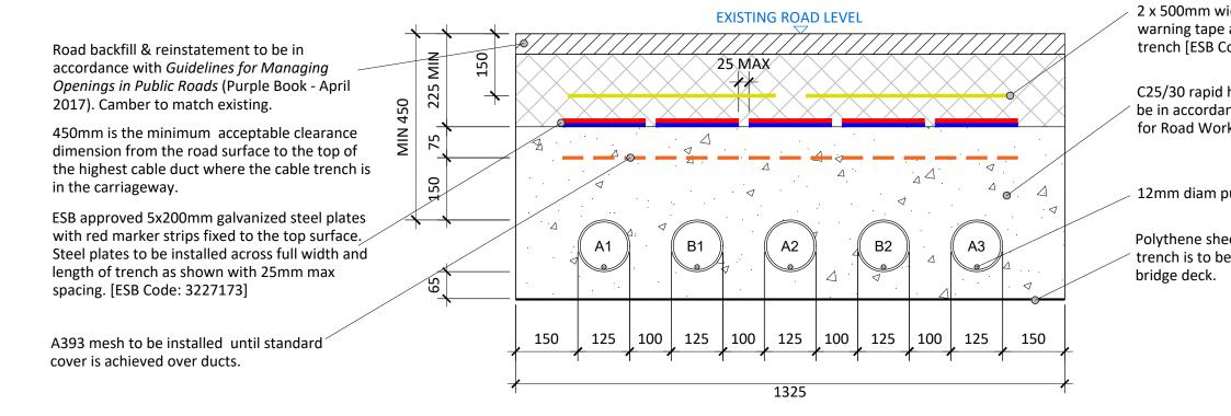
A = 125mm: Outer Diameter HDPE ESB Approved Duct, SDR=17.6 (Power) B = 125mm: Outer Diameter HDPE ESB Approved Duct, SDR=17.6 (Comms)
